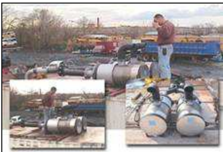
Installation of an active diesel particulate filter on a generator (above) and a diesel particulate filter on a tower crane (right).
